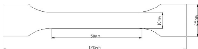
Figure 1. Schematic diagram of the samples for mechanical properties measurement.
